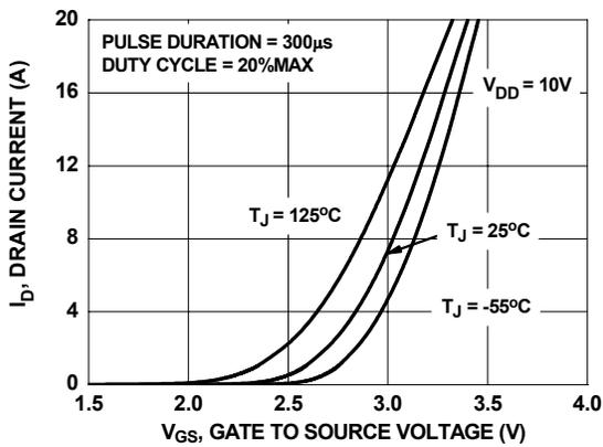
Figure 5. Transfer Characteristics
