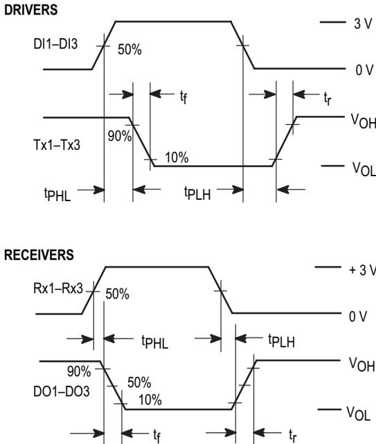
Figure 2. Switching Characteristics
