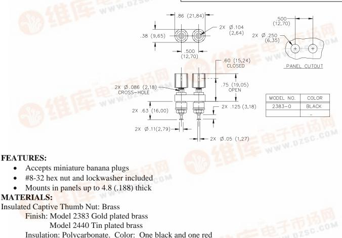
Mounting Base: Black Polycarbonate. Marking: "POMONA ELECTRONICS CALIF. Insulator: Polycarbonate. One black and one red
