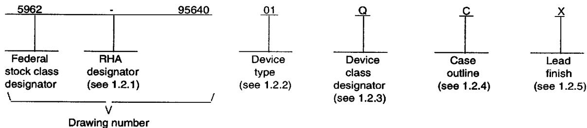
1.2.1 **RHA designator.** Device classes N, Q, and V RHA marked devices meet the MIL-PRF-38535 specified RHA levels and are marked with the appropriate RHA designator. Device class M RHA marked devices meet the MIL-PRF-38535, appendix A specified RHA levels and are marked with the appropriate RHA designator. A dash (-) indicates a non-RHA device.
