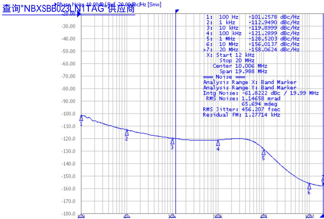
Figure 3. Typical Phase Noise Plot
