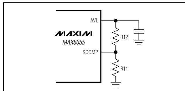
Figure 6. Resistor-Divider for Setting the Slope Compensation
