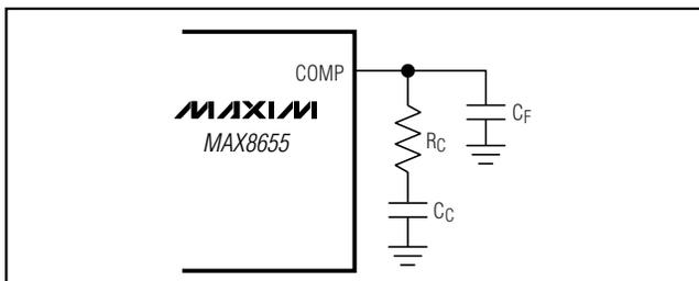
Figure 9. Compensation Components
