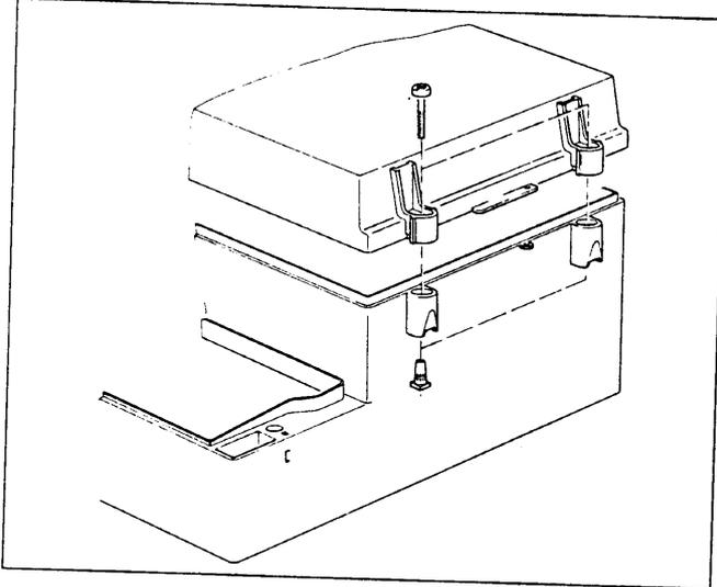
With this threaded sleeve screw kit the transparent lid can be screwed to the enclosure with or without a hinge.
