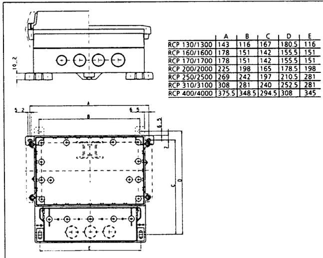
To mount the enclosure on a wall. The enclosure does not need to be opened. Will fit all RCP models:
