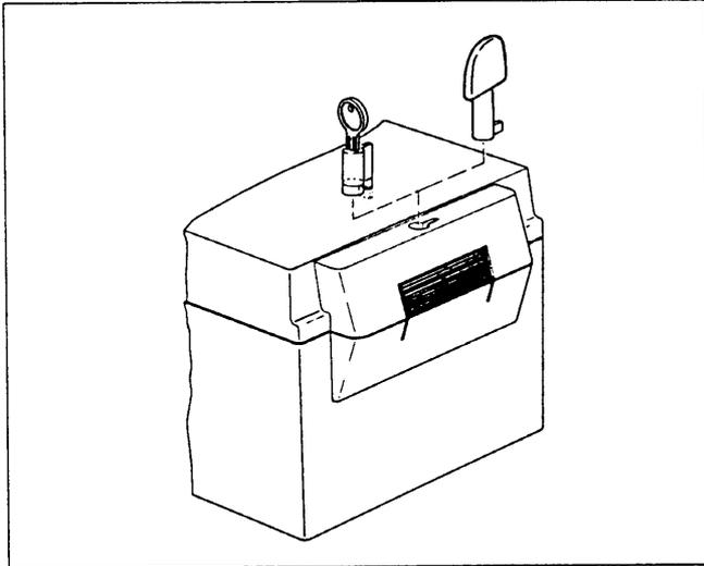
The cylinder lock or hand latch can be fitted later to the opening in the fastening. If a blanking plug is attached, this can easily be loosened from the rear and pressed out.
