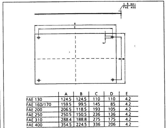
The aluminium front plates are anodized, 1 mm thick, and their dimensions match those in the RC enclosure series. Please note: front plates up to 3 mm thick can be inserted in RCP enclosures.
