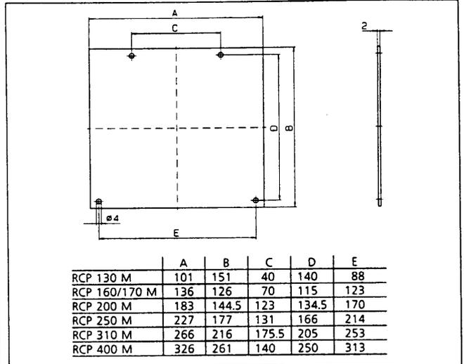
These mounting plates (laminated paper) are pre-punched for attachment in the enclosure and the terminal compartment. The mounting plates in the RC series can also be inserted in the RCP model.
