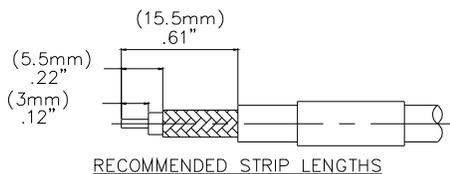
4. INSERT CONTACT PIN ONTO CABLE'S CENTER CONDUCTOR SO THAT IT IS FLUSH TO DIELECTRIC, CRIMP OR SOLDER CONTACT FIRMLY.
