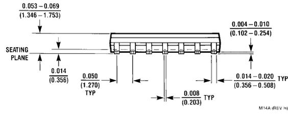
**14-Lead Small Outline Integrated Circuit (SOIC), JEDEC MS-120, 0.150" Narrow
