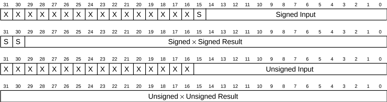
Figure 39. 16 x 16 Multiplier Data Formats
