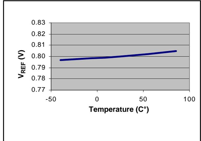
Figure 9. V<sub>REF</sub> vs. Temperature
