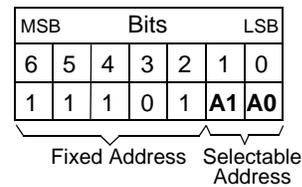
Figure 21. Address Bit Definition for 7-Bit Address
