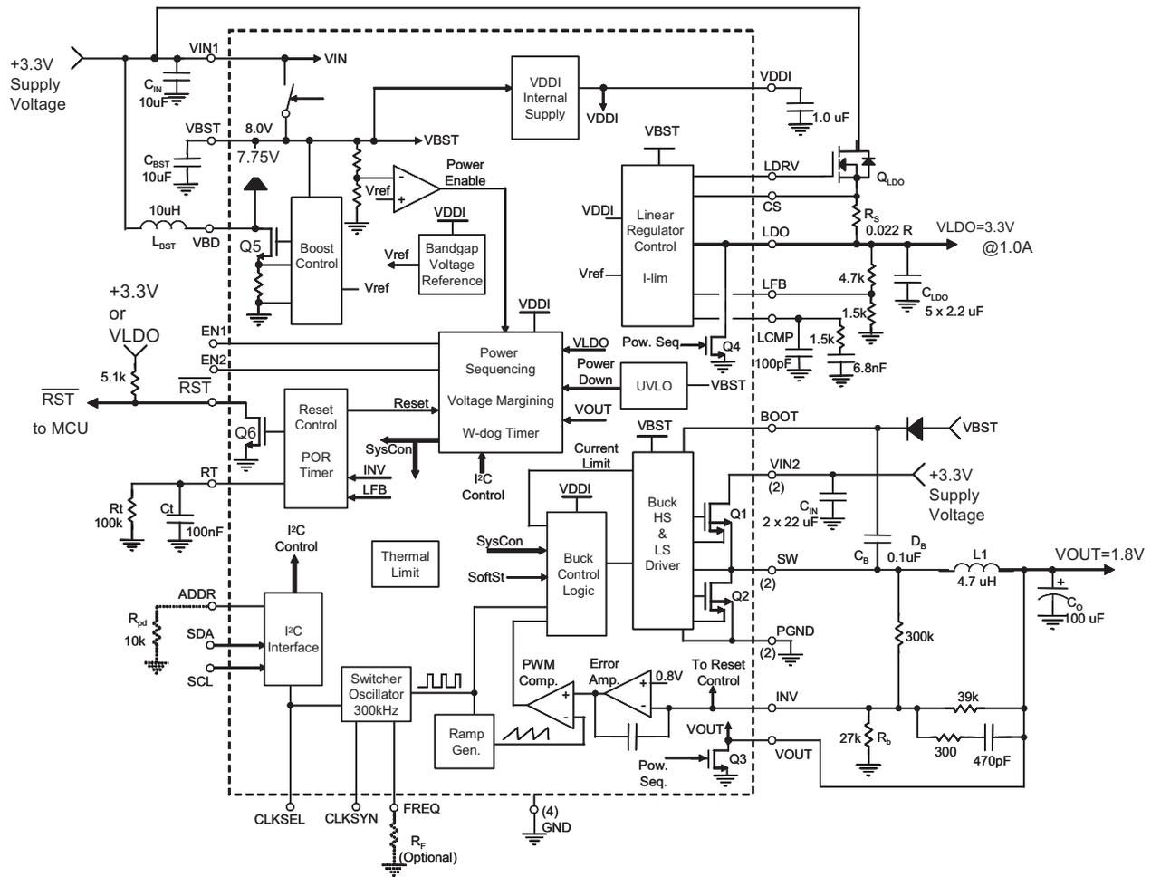
Figure 33. Simplified Block Diagram and Basic Application
