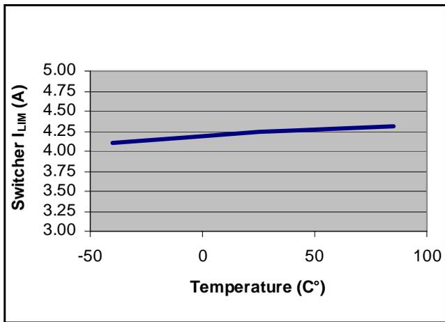
Figure 8. Switcher I<sub>LIM</sub> vs. Temperature
