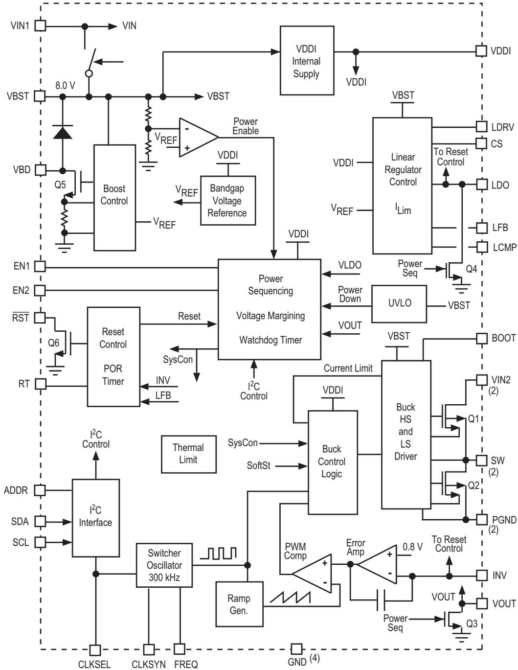
Figure 2. 34702 Simplified Internal Block Diagram
