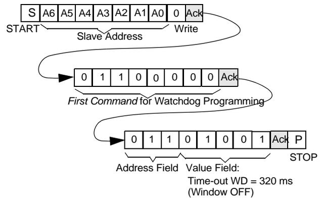
**Figure 26. Data Transfer Example - Watch Dog Timer Setting.**
