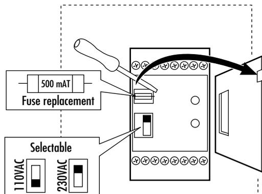
Mount in enclosure to a min of IP 54.
