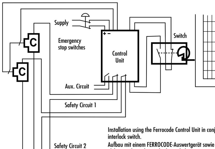
**NOTE:** Electromechanical switches require 1 N/O & 1N/C contacts for connection to the Ferrocode control unit.
