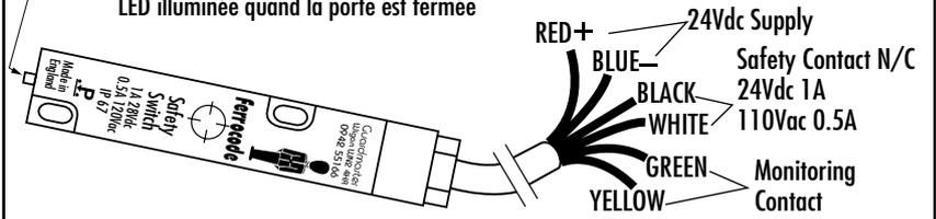
Safety contacts, one normally closed when the guard is closed and power is on.
