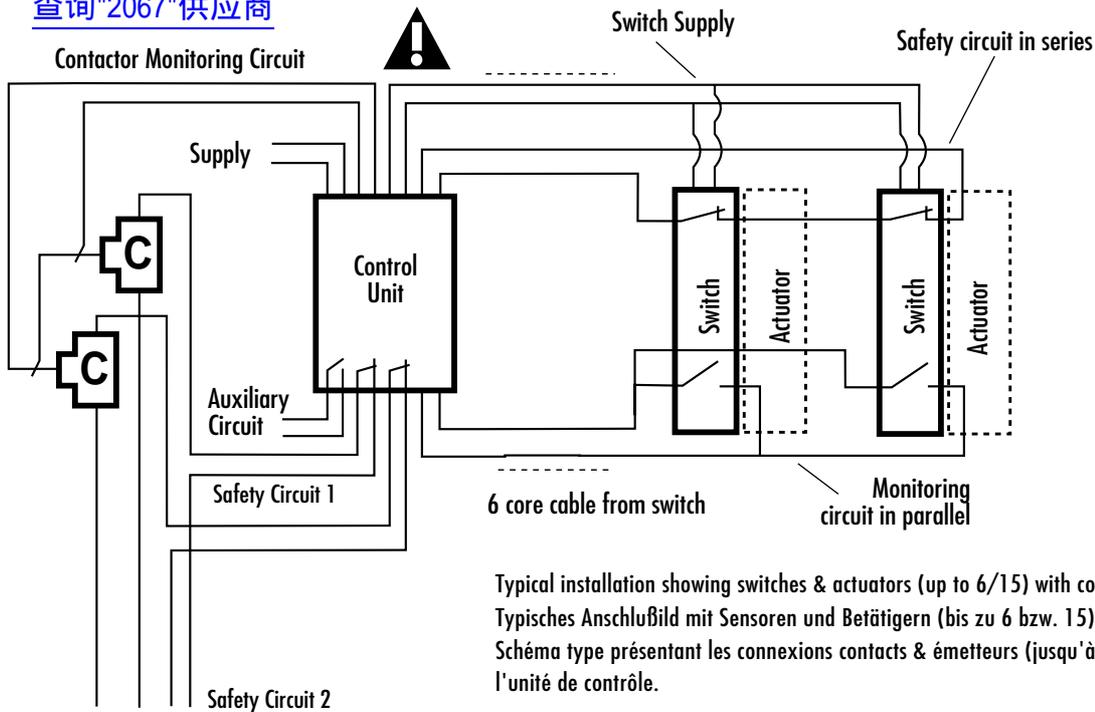
**NOTE:** With a multiple switch configuration it is recommended that as part of a regular inspection regime, each guard door is opened and closed in turn. This will enable detection of all single faults and prevent an accumulation of faults occurring on switches which are rarely operated, (or are always operated when another guard on the system is opened).
