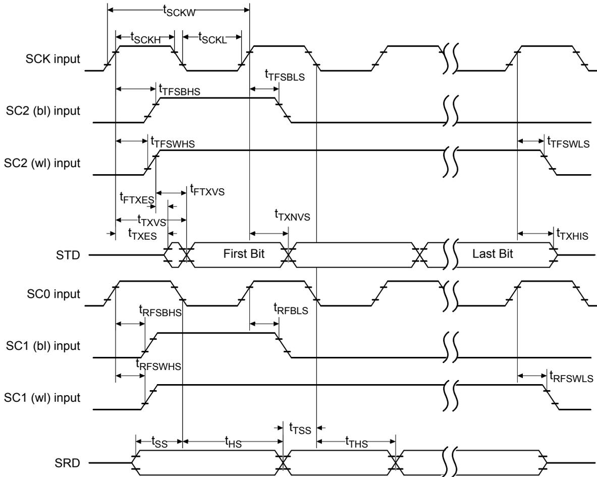
Figure 4-30 Slave Mode Clock Timing
