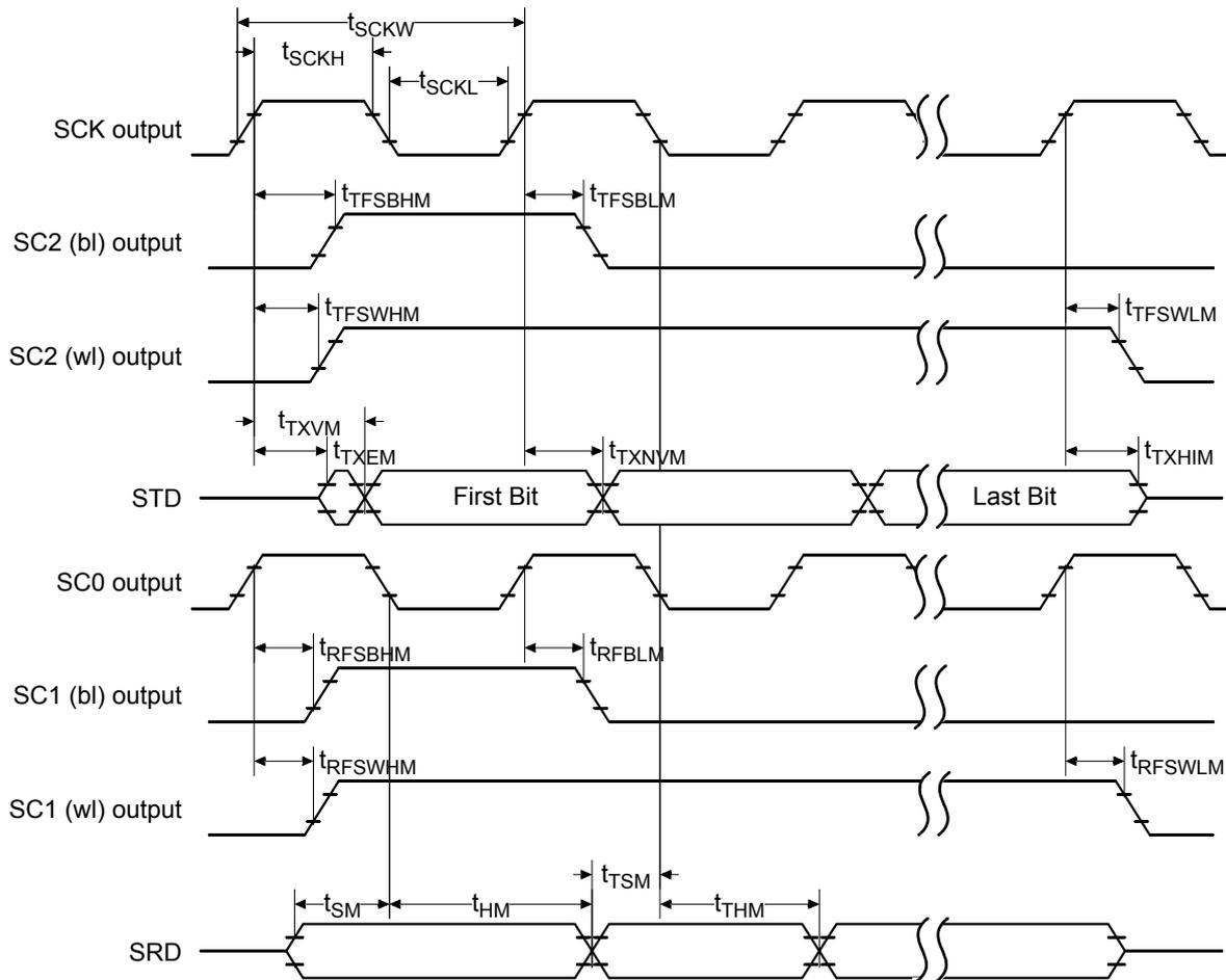
Figure 4-29 Master Mode Timing Diagram
