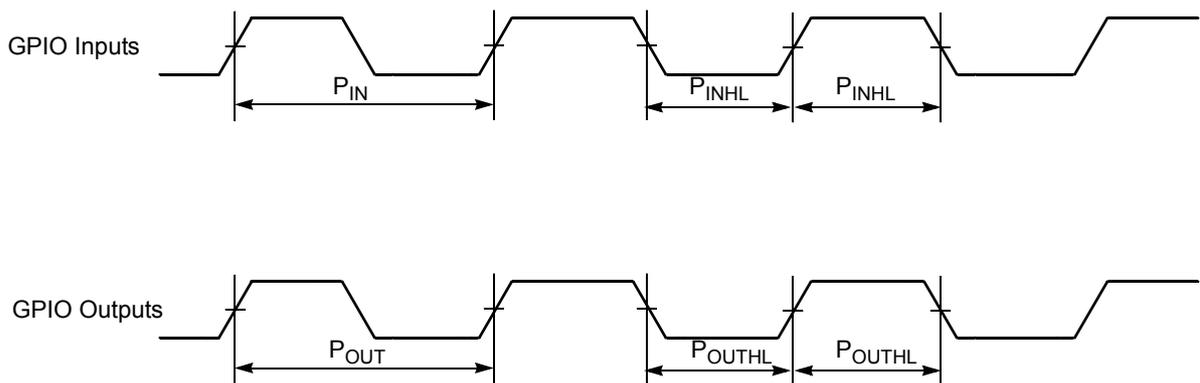
**Figure 4-37 GPIO Timing**
