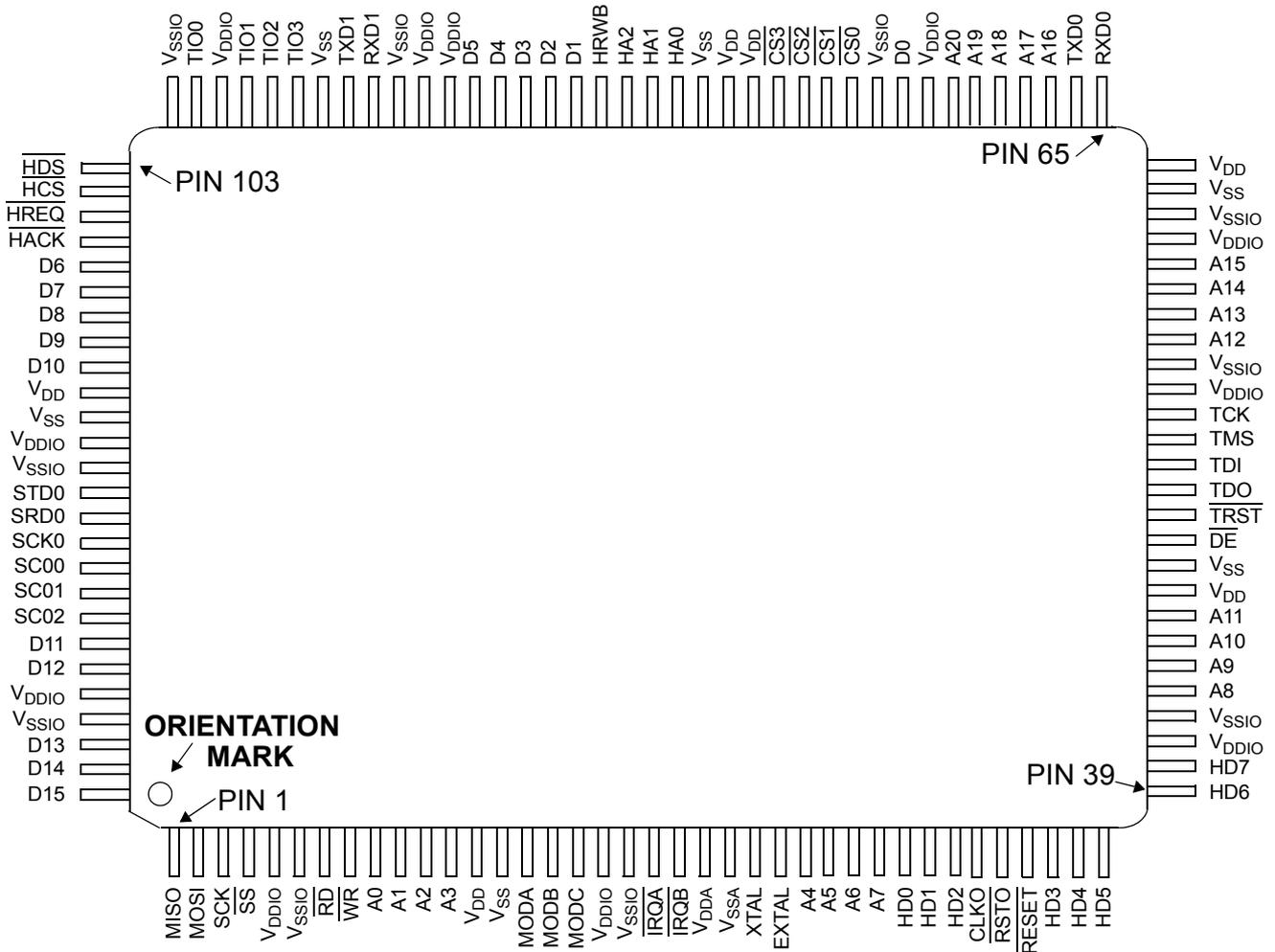
Figure 5-1 Top View, 56854 128-pin LQFP Package
