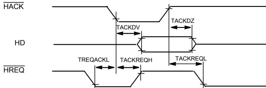
Figure 4-18 Controller-to-Host DMA Read Mode
