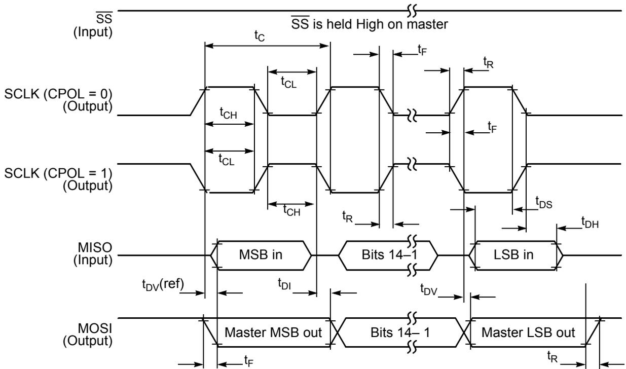
Figure 4-25 SPI Master Timing (CPHA = 1)
