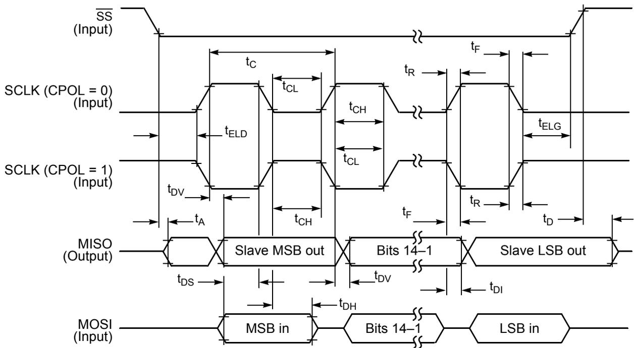
Figure 4-27 SPI Slave Timing (CPHA = 1)
