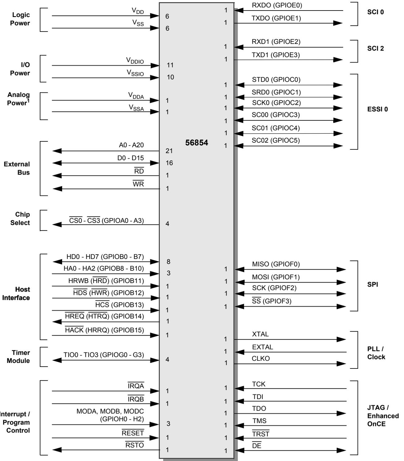
Figure 2-1 56854 Signals Identified by Functional Group<sup>2</sup>
