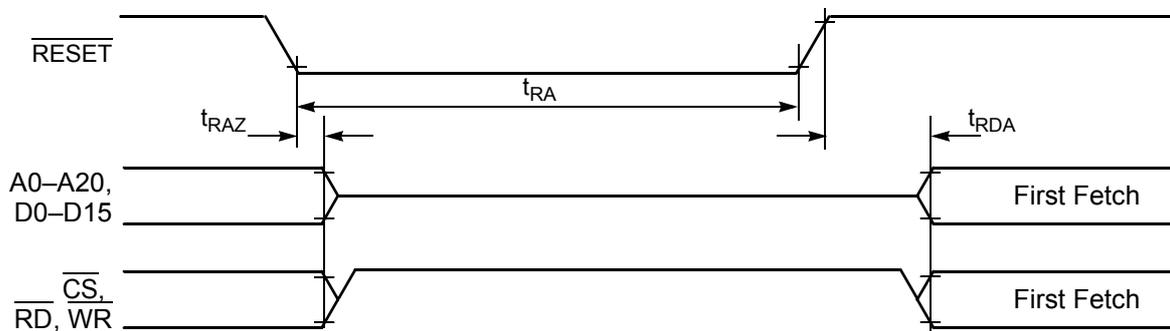
**Figure 4-12 Asynchronous Reset Timing**
