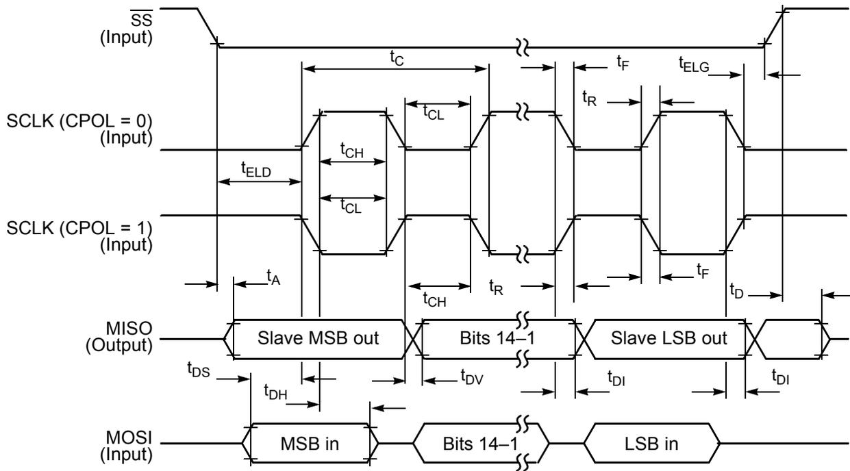
Figure 4-26 SPI Slave Timing (CPHA = 0)
