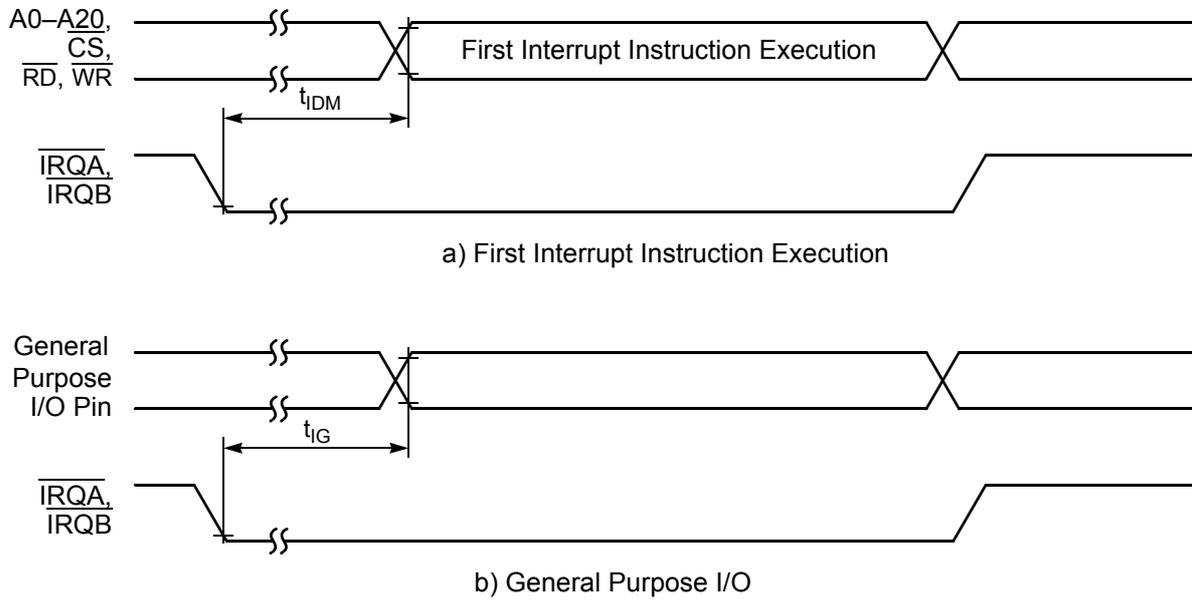
Figure 4-14 External Level-Sensitive Interrupt Timing
