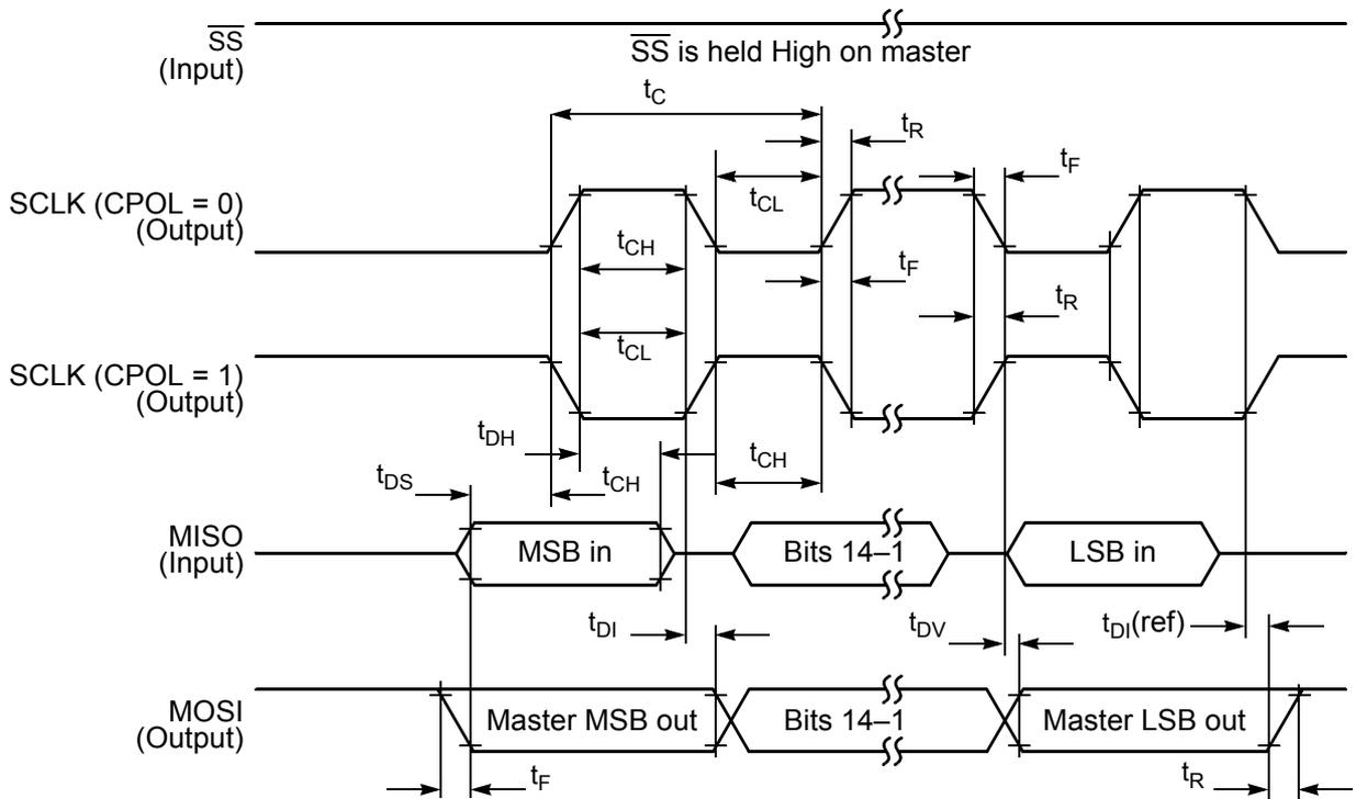
Figure 4-24 SPI Master Timing (CPHA = 0)
