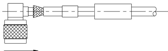
7. CRIMP FERRULE WITH APPROPRIATE CRIMP TOOL. SLIDE SHRINK TUBING OVER CRIMP AND SHRINK.
